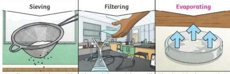
Smaller materials are able to fall through the holes in the sieve, separating them from larger particles.
